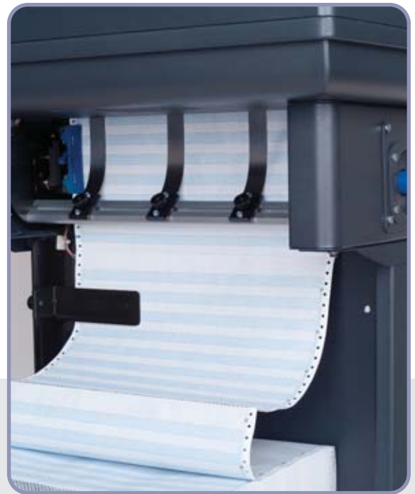
Push tractor system eliminates forms loss
