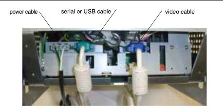
• Connect the power cable to the AC connector on your touchmonitor. To protect your equipment against risk of damage from electrical surges in the power line, plug the touchmonitor's power cord into a switched surge protector, and then connect the surge protector to a grounded (three-pronged) AC electrical outlet.
