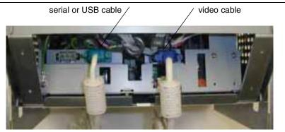
• Depending on your monitor, connect either the serial or USB touchscreen cable. Connect one end to the appropriate port on the back of your computer. Connect the other end of the cable to the touchscreen connector on your touchmonitor. The touchscreen cable connectors should fit snugly into the connectors on your touchmonitor and computer. Secure the cable by turning the thumbscrews on each connector.
