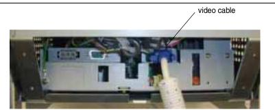
• Connect one end of the video cable to the video connector on your PC and the other end of the cable to the video connector on your monitor. Secure the cable by turning the thumbscrews on each connector.
