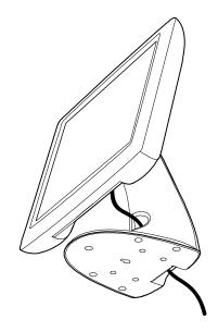
• Feed the cables through the cable port holes. Do not remove the rear cover.
